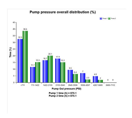
The diagram describes Pump outlet pressure of 2 Pumps distribution.
