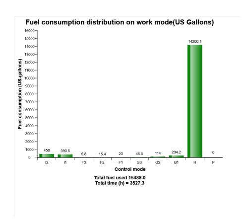
The diagram describes the amount of fuel consumed per engine speed mode distribution.
