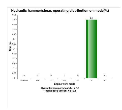
The graph describes the operating hours (%) for hydraulic hammer/shears on each engine control mode .
