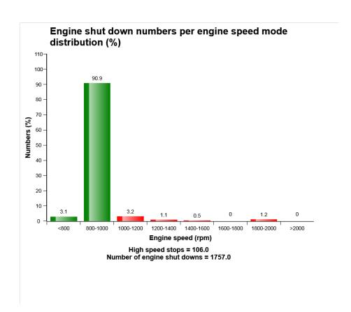
The diagram shows the number of stops at high idle (I1 ~ P mode).
