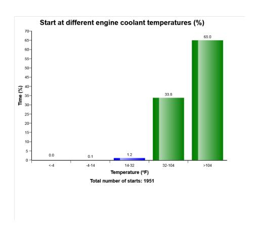
The graph shows the distribution of engine coolant temperature, at the starting moment.
