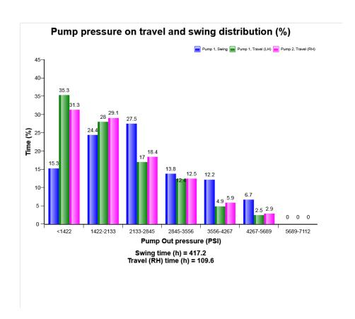
The diagram describes Pump outlet pressure of 2 Pumps for travel and swing operation distribution. In case operator use several operations at the same time, this pressure distribution for travel and swing operation can be different from actual operating pressure distribution for travel and swing operation in field.
